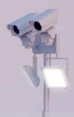
The Harbinger solution is a system designed to assist in the detection of vehicles in a sterile or closed off area. The detection of the vehicles in these areas is to provide early warning and detection of vehicles that could potentially be utilised for a Vehicle as a Weapon attack (VAW).
